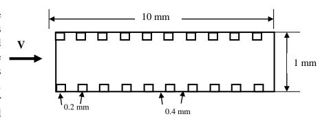
dispersion and deposition of particles in the range of 0.01 to  $10~\mu m$  from point sources located at three locations in the duct inlet. Also, evaluate the deposition of particles for a uniform inlet concentration.
