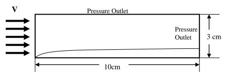
velocity profiles, boundary layer thickness as a function of distance, and  $C_{\rm f}$  and  $C_{\rm D}$ . Use an inlet velocity of 0.02 m/s and assume the flow is laminar.
