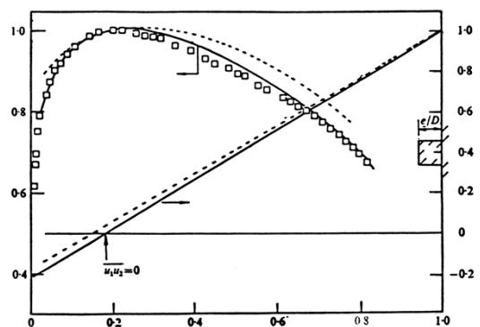
**Mean Velocity and Turbulence Shear Stress**
