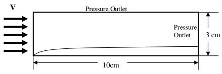
velocity profiles, boundary layer thickness as a function of distance, and  $C_f$  and  $C_D$ . Use an inlet velocity of 0.02 m/s and assume the flow is laminar. Compare your findings with the theoretical predictions.
