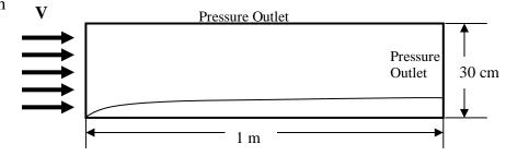
boundary layer thickness as a function of distance, and C<sub>f</sub> and C<sub>D</sub>.
