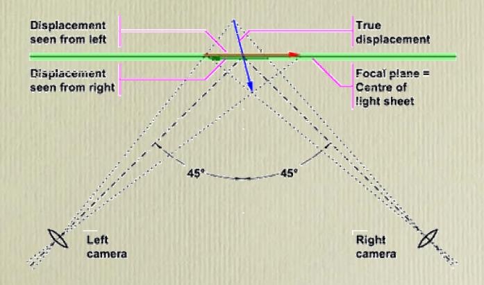
Make measurements of flow through the measurement plane.
