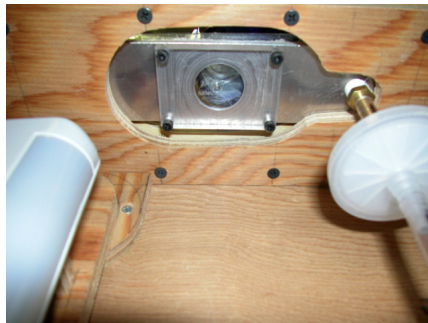
Figure 2: The four allen head bolts holding the slide to the channel should only be finger tight. These must be removed to access the test section.
