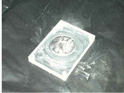
Figure 5: This slide probably has too many particles on it. The pipe cleaner can be used to brush a few particles off the surface or to spread the particles more evenly.
