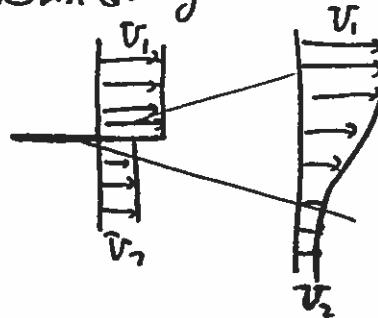
2. Using  $\frac{u}{U_\infty} = 1 - \exp\left\{-ay \over \delta\right\}$  as an approximate expression for the velocity distribution in the boundary layer over a flat plate, determine  $\delta$ ,  $\delta^*$  and  $\theta$ . Find 'a' such that  $\delta$  becomes identical to the exact solution of the Blasius equation.
