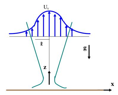
$$U\frac{\partial W}{\partial x} + W\frac{\partial W}{\partial z} + \frac{\partial}{\partial x}\overline{u'w'} = \frac{g_0\overline{T}}{T_0}$$
